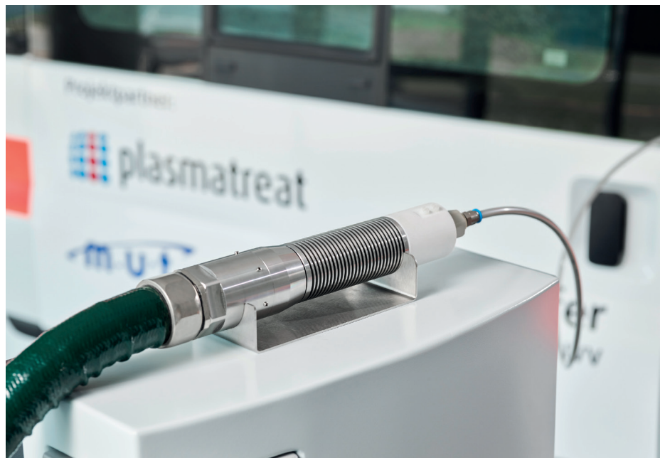
Fig. 4: The new developed nozzle can reduce the bacterial load by a factor of one million, which meets the requirements for sterilization. Photo Plasmatreat
