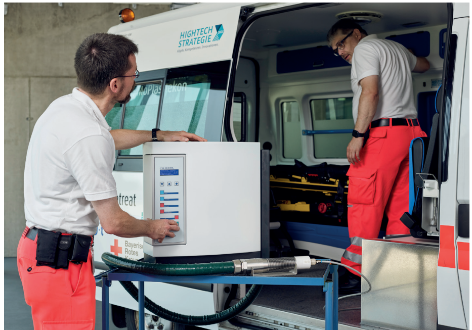
Fig. 1.: The newly developed mobile plasma decontamination system (MoPlasDekon) can disinfect the interior of the entire ambulance during emergency situations without using chemicals.
