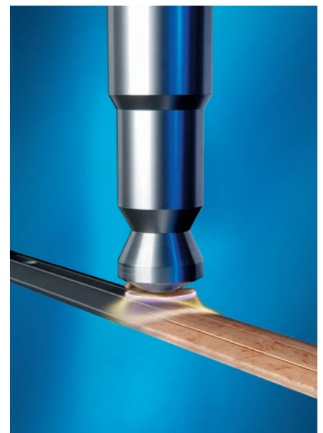
Fig. 5: Wrapping of aluminum trims: Pretreatment using AP plasma jet technology is not only much faster than dipping processes, it is also environmentally friendly and far more cost-effective (Photo: Plasmatrete)
