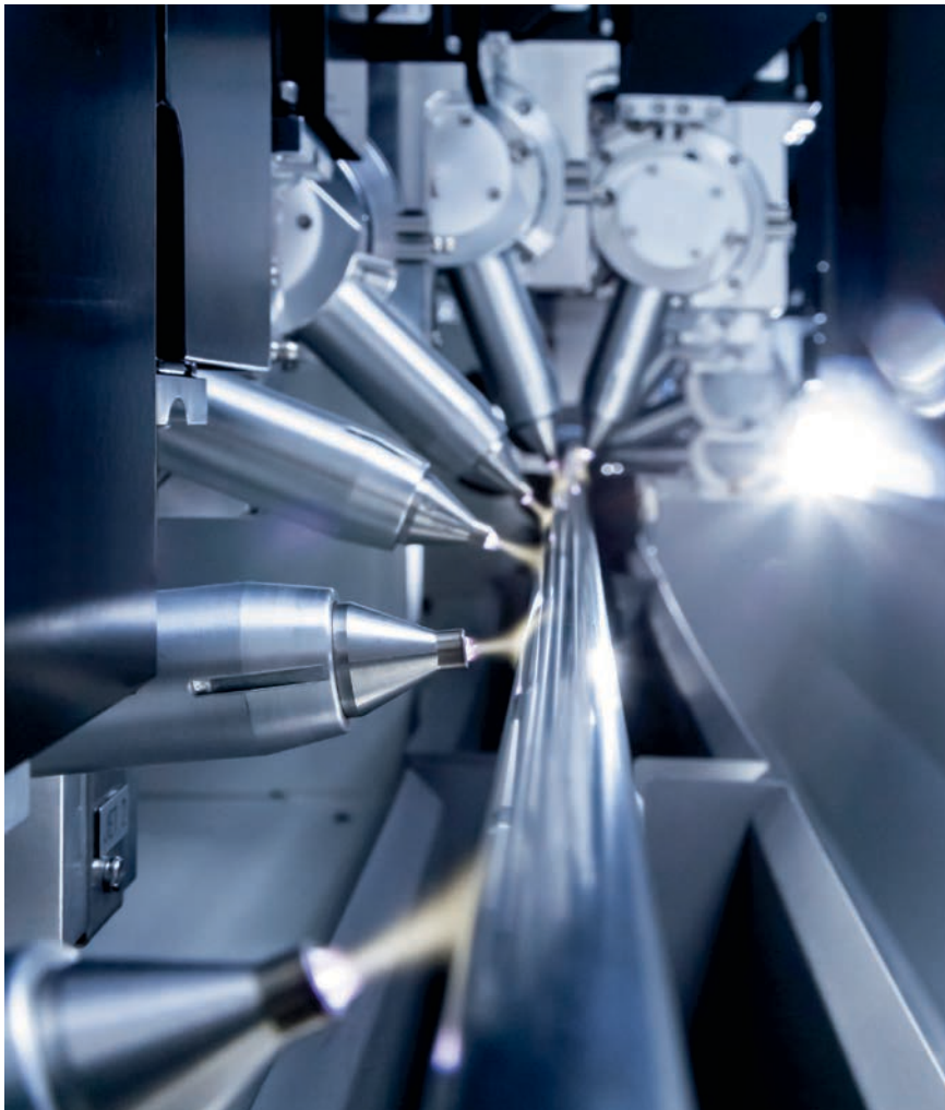
Figure 2 > Nozzle combination: Inline plasma treatment in the continuous extrusion process for EPDM profiles
