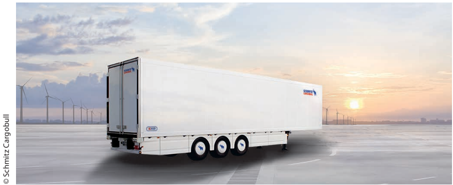
Figure 4 > The panel surfaces of the self-supporting refrigeration system are pretreated with environmentally friendly Openair-Plasma to enhance the durability and tightness of the adhesive bond.
