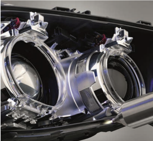
Figure 6 > Hella has used Openair-Plasma for over 20 years as a pretreatment in the process of bonding polycarbonate lenses to polypropylene housings.
