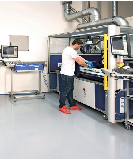
Fig. 6: Environmentally friendly and cost-effective: Plasma system (right) and bonding station (left) are immediately opposite one another. The housing is bonded immediately after the Openair-Plasma® pretreatment (Photo: Plasmatreat)
