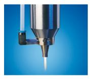
The PlasmaPlus process makes use of a precursor to apply area-selective, nanofine functional coatings to material surfaces (Source Plasmatreat)
