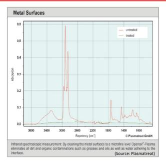
surface energy which gives them their adhesive characteristics can be compromised by layers of oxides, dust deposits, grease and oils or other contaminants. This is where the microfine cleaning action of the plasma comes into play, revealing once again the high level of surface energy already present in the substrate. Materials can be further processed immediately after cleaning and activation with AP plasma.
