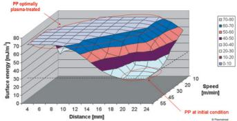
Treatment renders the plastic surface polar and increases the surface energy to >72mJ/m² (72 dyne) with a large process window (Source: Plasmatreat)
