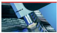
Environmentally friendly pretreatment in lightweight automotive construction: Prior to bonding, a CFRP surface is cleaned to microfine level and activated with Openair-Plasma to ensure long-time stable adhesion (Photo: Plasmatreat GmbH)
