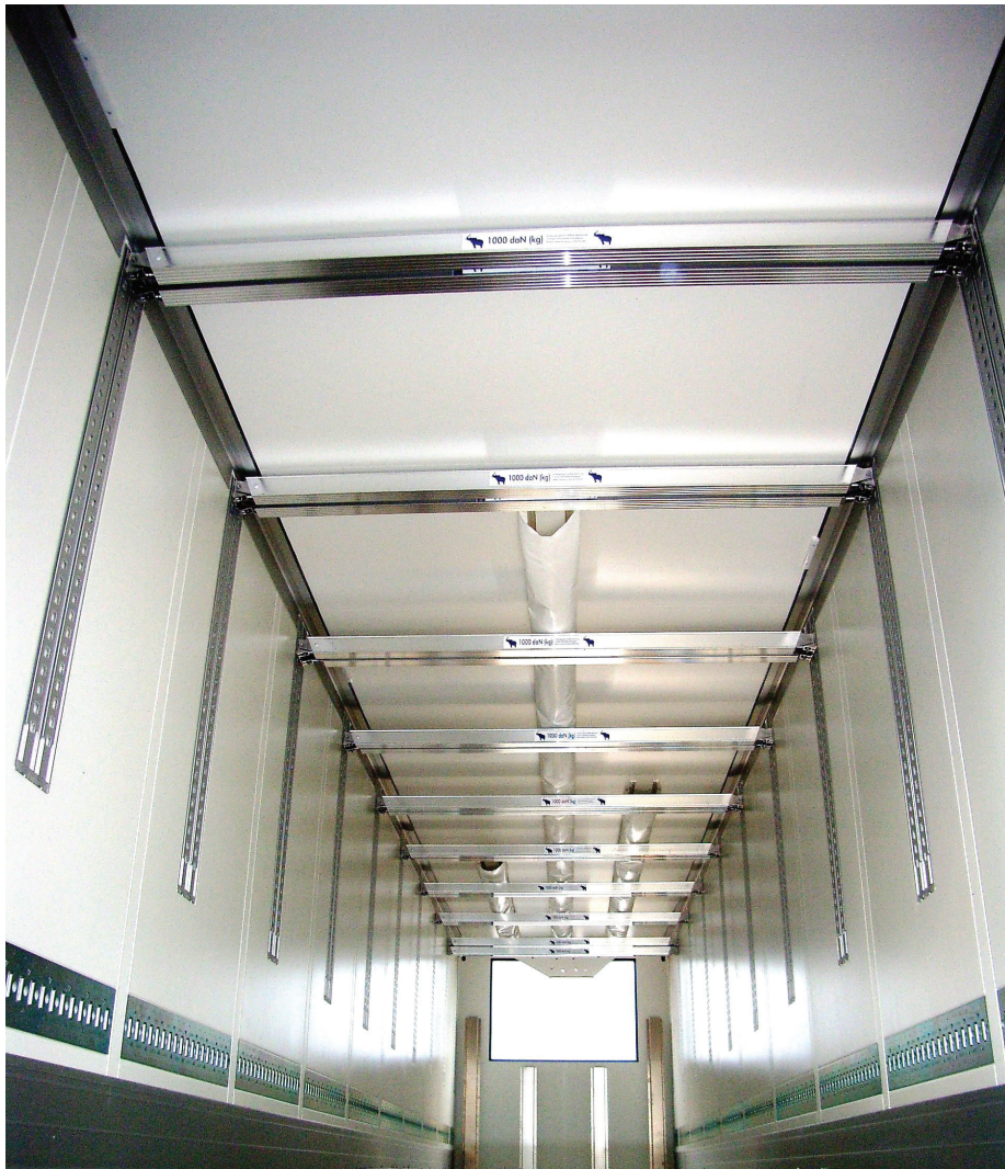
Fig. 7. Photo Blue Rondo International The load securing rails are flush-mounted in the metal outer skins of the panels. Plasma pretreatment ensures strong adhesive bonds.
