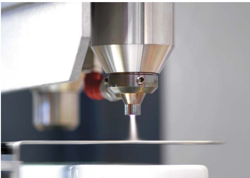
Fig. 1: The chemical-physical Plasma-SealTight process enables the area-selective deposition of functional nanocoatings in milliseconds and thus the creation of covalent bonds between different materials. (Pictures: Plasmatreat GmbH)
