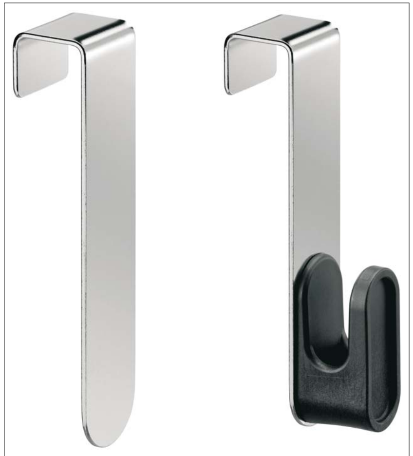
Fig. 2: The metal part (left) can be overmolded with the thermoplastic compound (right) immediately after atmospheric pressure plasma coating to produce a strong joint.
