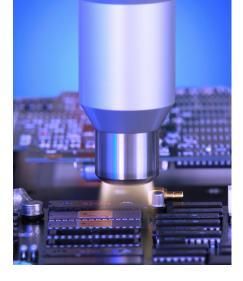
lity, was also rejected. The final method under consideration was a low-pressure plasma treatment; a highly effective activation process, but not suitable for this purpose because the vacuum would have drawn the fluid out of the wet electrolytic capacitors contained in the SMD assembly. A solution to the problem still seemed a very long way off.
