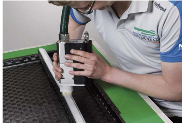
Fig. 11: Plasma treatment of the rigid foam rib using a hand-held rotary nozzle. (Photo: Plasmatreat)
