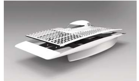
Fig. 4: Assembly of the different car body layers (Photo: Punch Powertrain Solar Team)
