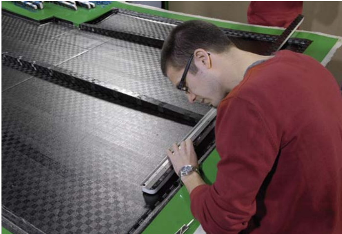
Fig. 10: Production manager Dokus Soetemans measures and marks the adhesive surface with millimeter precision. (Photo: Plasmatreat)
