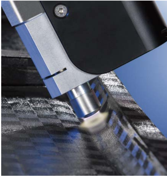
Fig. 7: Pretreating the CFRP surface with an «Openair» plasma rotary nozzle brings about simultaneous microfing cleaning, electrostatic discharge and strong activation of the plastic significantly enhancing its wettability and adhesive properties. (Photo: Plasmamatreat)
