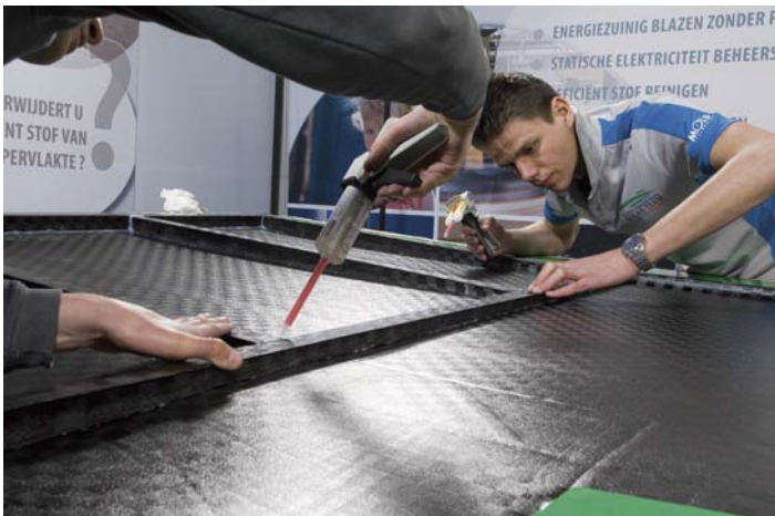
Fig. 12: Immediately after plasma treatment, the rib is bonded with a 2-component epoxy adhesive. (Photo: Plasmatreat)
