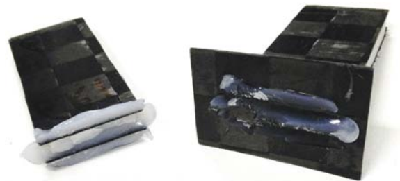
Fig. 9: Cohesive fracture in the adhesive after plasma treatment (Photo Punch Powertrain Solar Team)
