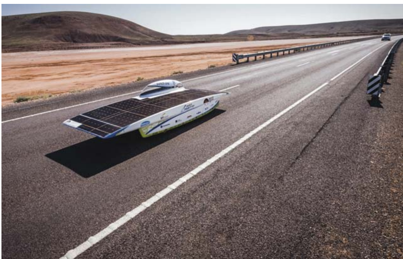
Fig. 1: Powered only by the sun: The energy-efficient «Punch One» solar car at the World Solar Challenge rally in Australia. The plasma bonding process reduced the weight of the CFRP body by several kilos. (Photo: Punch Powertrain Solar Team)
