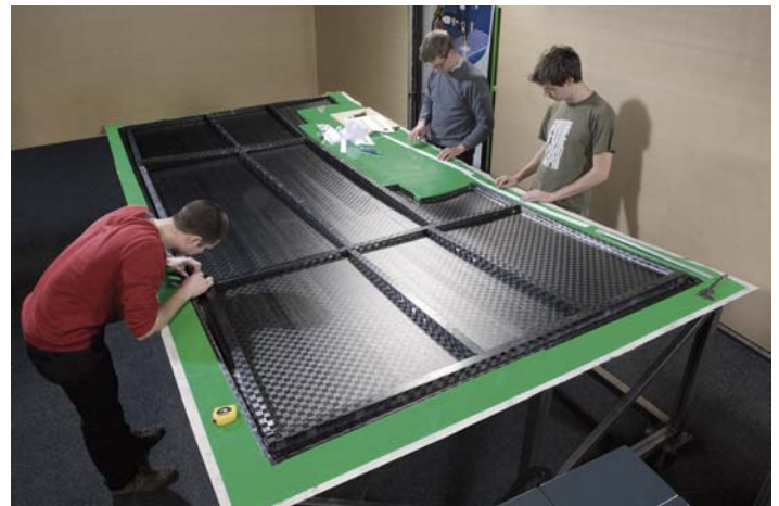
Fig. 13: The monocoque outer shell receives its final stiffening rib. (Photo: Plasmatreat)
