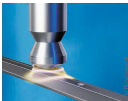
Fig. 4: AP plasma treatment of aluminum trims before painting: The deep-pore cleaning action of the rotating plasma beam reveals the high surface energy already present in the aluminum.
