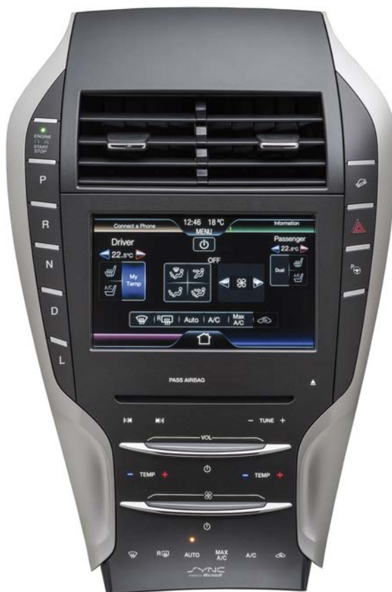
Fig. 1: The so-called center stack is the heart of the central console. Only by using atmospheric pressure plasma could a bubble-free bond between the sensitive PET touch foil and the new 3D control panel in the Ford Lincoln MKZ be ensured. (Photo: Preh)
