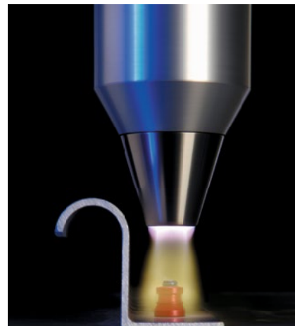
Proximity of the nozzle to the treated surface and speed of treatment are the fundamental parameters of the plasma process.
