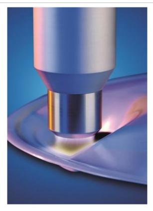
DÜSSELDORF, GERMANY — Plasmatreat GmbH presented a live demonstration at K 2013 of its new Openair atmospheric plasma treatment unit designed for fully automated EPDM profile treatment processes.
