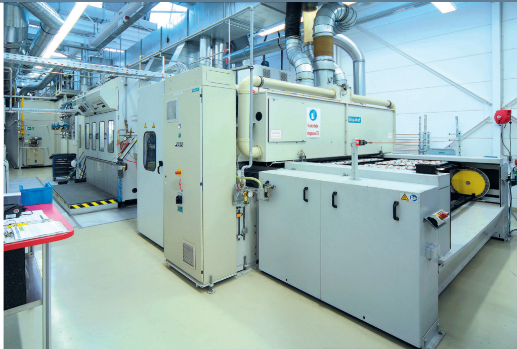
Fig. 1 – The Openair plasma system (3rd unit from the front) takes up only one metre of a painting line with an overall length of 25m
