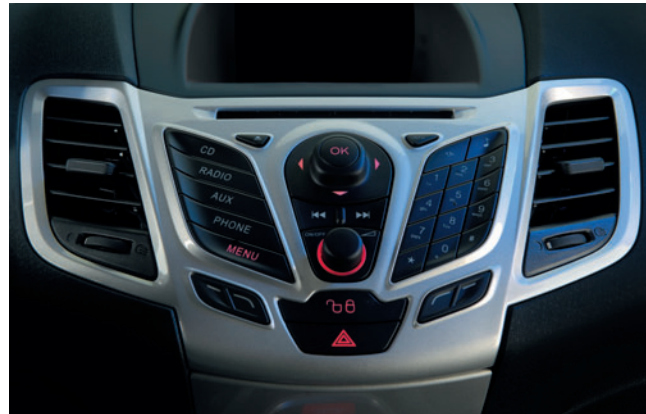
Figure 1. The integrated control panel (ICP) forms the centrepiece of the dashboard. The plastic switches are pretreated with atmospheric plasma before painting to ensure a flawless finish and an adhesion that will last for years
