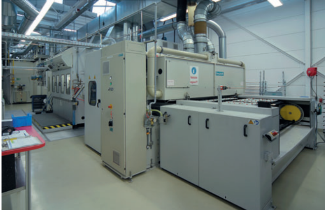
Figure 2. The Openair plasma system (3rd unit from the front) takes up only one metre of a painting line with an overall length of 25 m
