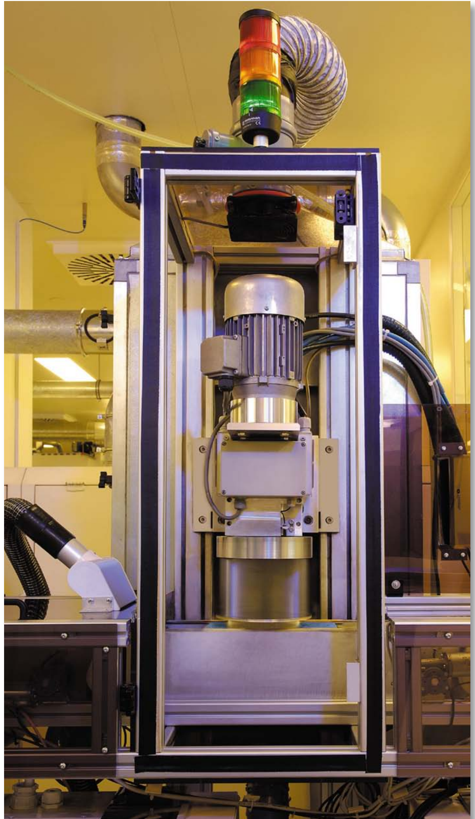
Figure 7: The circuit boards undergo a continuous process, via the plasma system, through to the screen printing plant. The space-saving plasma plant serves four screen printing lines. (Plasmatreat)
