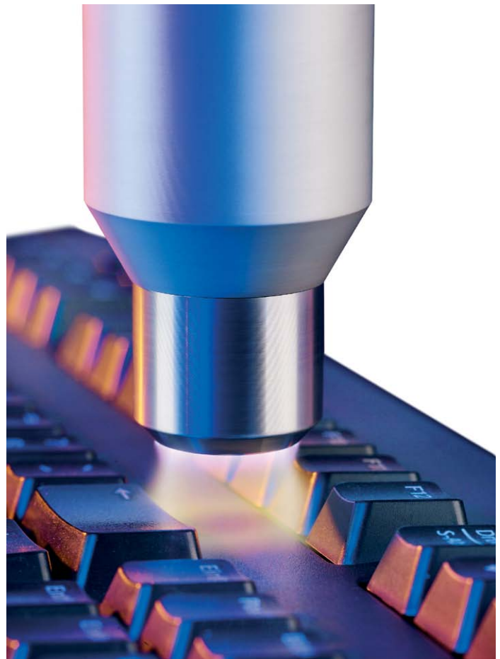
Figure 2. Electrostatic effects are the principal cause for the adhesion of dust. Atmospheric plasma-jet treatment allows extremely efficient cleaning before decorating.
