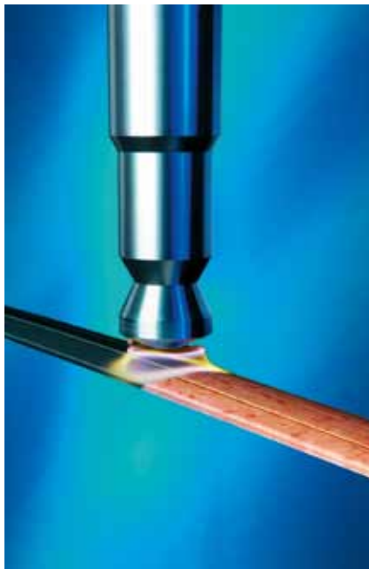
Aluminium strips before wrapping chromating is completely replaced by atmospheric plasma treatment
