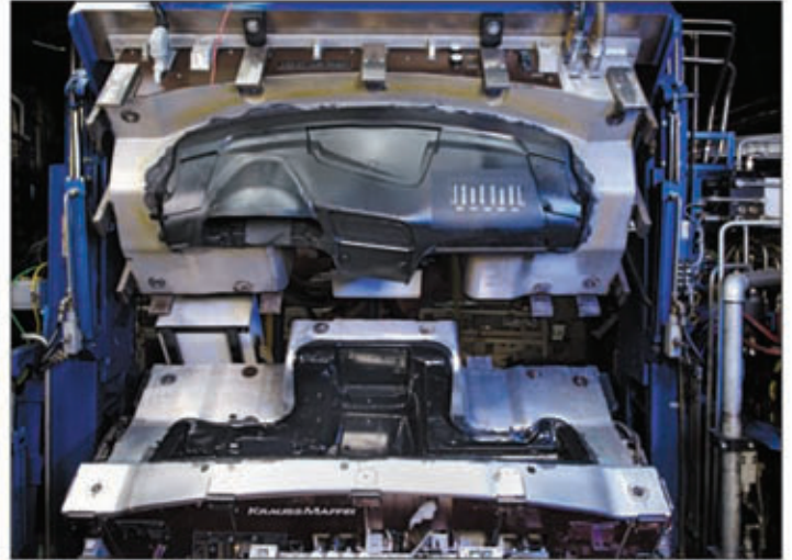
Figure 3: The foam installation appears like a giant sandwich toaster when opened. The PUR foam will be applied on top of the slush skin in the lower mould. After closing the installation the foam spreads equally between the PP-board (top) and the skin, bonding both together.
