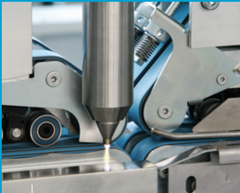
The 'cold' plasma beam ensures perfect bonding in high-grade folding boxes and leaves no visible traces on the surface.
