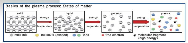
Plasma technology doesn't stop at the gaseous state of matter: If by means of electric discharge additional energy can be fed into the material, the electrons gain more kinetic energy and leave their atomic shells.
