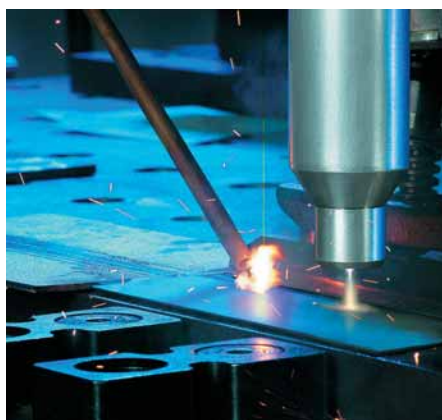
7 Cleaning with Openair plasma prior to MIG welding
