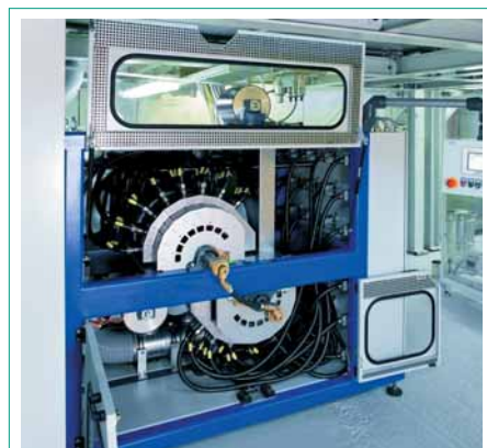
6 A world first: Use of plasma in the coil coating process at Griesser. Large volumes of wet chemicals are rendered superfluous by the plasma treatment
