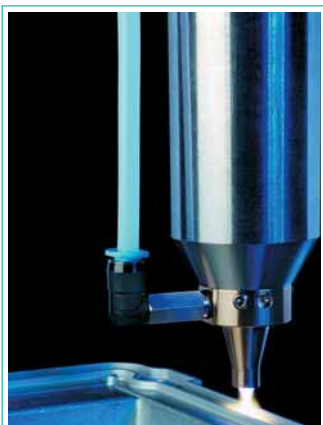
4 Coating the groove region of an aluminium housing for electronics
